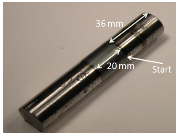
Figure 8-15 A wider cylindrical hardened surface obtained by AS technique.
