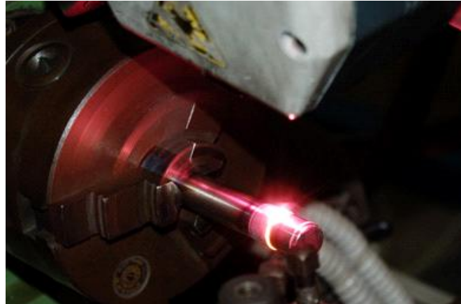
Figure 8-7 Apparent Spot technique applied in cylindrical surface.
