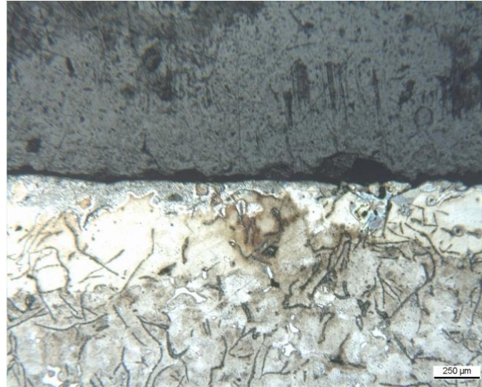
(b) Overlapped zone between 1 st and 2 nd tracks.
