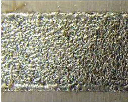
Figure 7-5 Melted surface obtained by small LD and low scanner head frequency.
