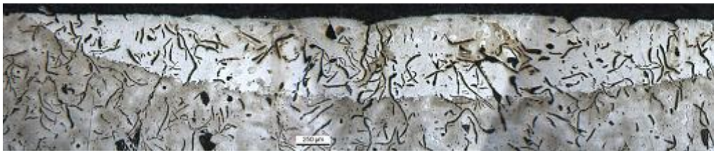
(a) Deformed top surface by melt
